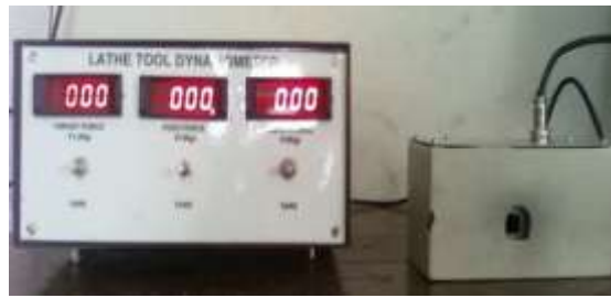
Figure 2 Strain gauge dynamometer
